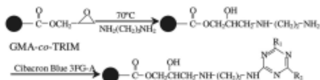
Fig. 1. Synthesis of Cibacron blue 3GA modified GMA-co-TRIM monolithic polymer.
